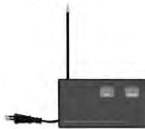
AFTRA02 is a transceiver with technological warning functions. It works simply placed on the floor and plugged to a 230V AC socket. A back up lead battery 6V 1,2 Ah is inside. Properly positioned, it allows to increase transmission range when necessary, because it repeats all AVE radio codes received. The device has a mains controller inside that can give a black-out alarm to a control panel or a dialler. Other external alarm devices can be connected in a NC/NO input terminals.
