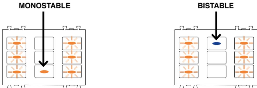
*From the roller shutter / pushbutton menu, push the P1 button once and choose the required function.*
