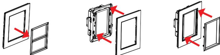
Remove the frame from the cover plate
