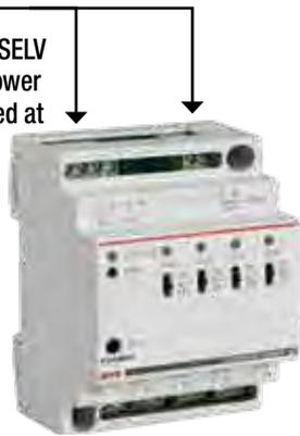
**Note:** the micro-two-way switches placed on the front, if in the ON or OFF position, manually force the output, while in the AUTO position the output follows the controls received from the bus.
