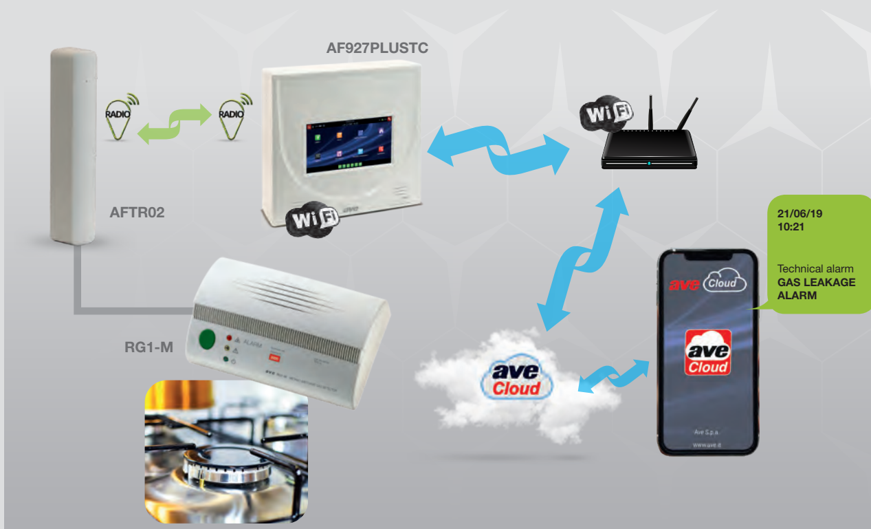
2) Example of PUSH notification for technical alarm (GAS leakage)
