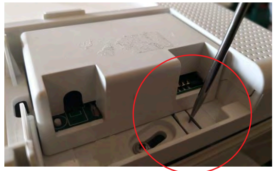
Should removal of the GSM module be required, press down on the catch securing the module using a pointed object.
