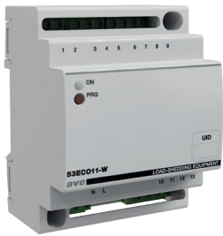
53ECO11-W Controllo carichi IoT per impianti monofase IoT load control for single- phase systems
